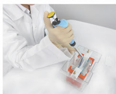
3-position tip ejector button (left/right handed users)
