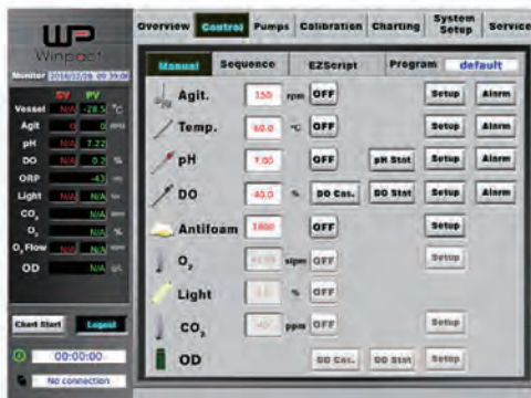
Control / Manual Manual operation, sequence or EZScript control (optional) of each parameter.
