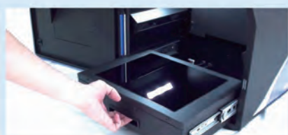
Pull out UV transilluminator
