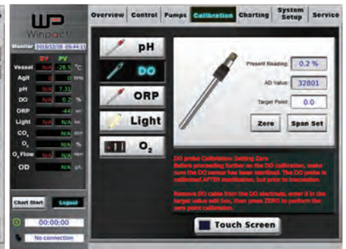
Calibration Easy sensor calibration with assisted menu
