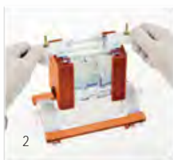
2 Transfer to casting base and tighten cams.
