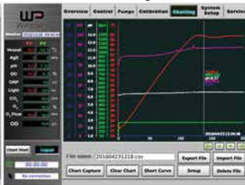
Real-time data recording and exporting during a fermentation process with image capture capability (NEW)
